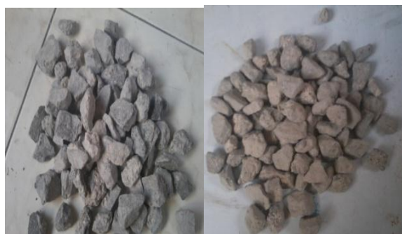
a) 20 min rolling b) 30min rolling Fig. 8: Recycled Aggregates after 20min and 30min Dry Rolling Proposed Method
