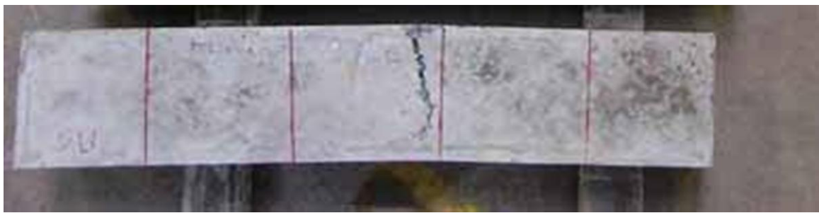
Fig. 4 Crack Patterns for Test Beam.
