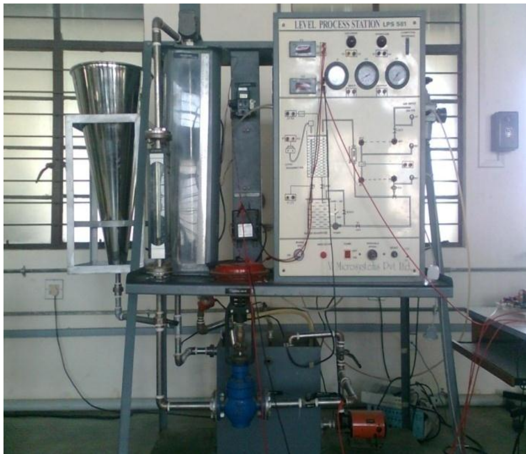
Fig. 6: Conical Tank Level Process Station
