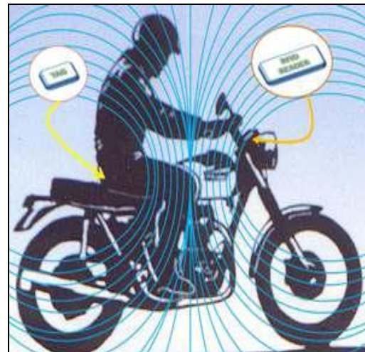
Fig. 2 look of immobilizer system in a bike
