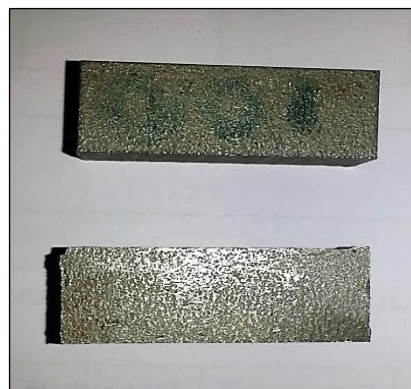
Fig. 2: Pieces of SS 304 Cut by AWJM.
