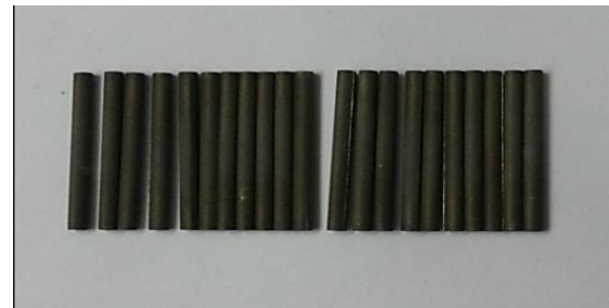
Fig. 4: Cr 3 C 2 NiCr Coated Ti6Al4V Specimens.
