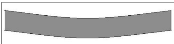
Fig. 7: Distorted Block after Welding.
