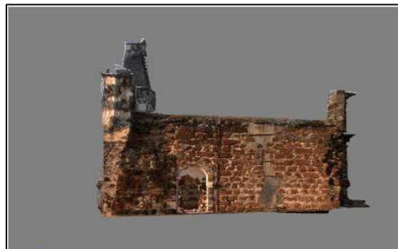
Fig. 5: 3D Visualised Model Using Terrestrial Laser Scanning [23].
