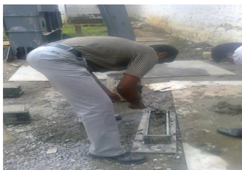
Fig 1: Casting of Specimens.
