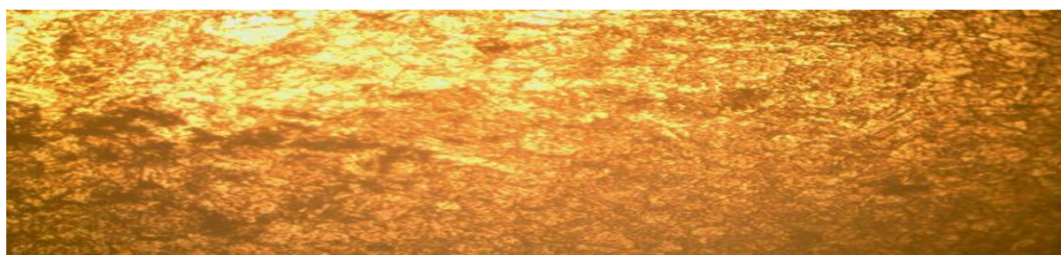
Plate 2a: Micrograph of Parent Annealed Austenitic Stainless Steel Showing Some Carbide Inclusion ( M_{23}Cr_6 ) Precipitates (Black), Delta Ferrite (White) in Austenitic Matrix (White Background) \times 100 .
