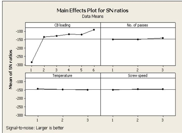
**Fig. 6:** Main Effects Plot for S/N Ratio Values of Volume Conductivity.
