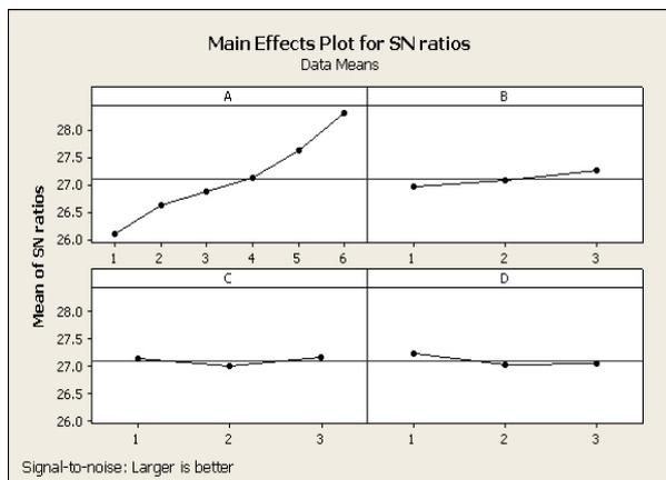
**Fig. 8:** Main Effects Plot for S/N Ratio Values of Microhardness.
