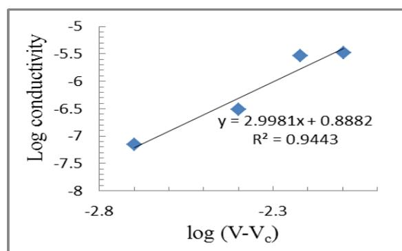
**Fig. 2: Log Conductivity v/s Log (V-V<sub>c</sub>) for Epoxy/CB Nanocomposite.****Table 3: Power Law Equation Parameters.**
