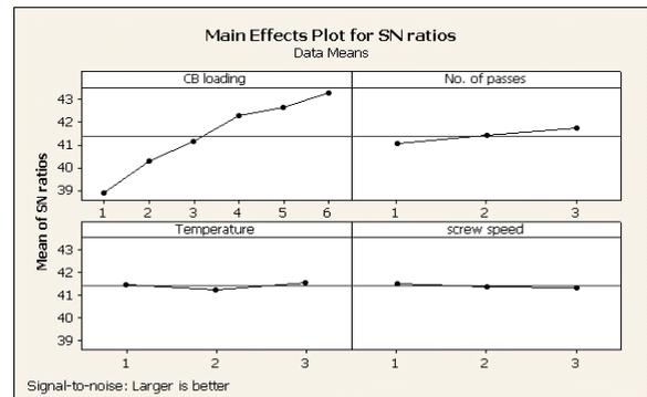
**Fig. 10:** Main Effects Plot for S/N Ratio Values of Impact Strength.
