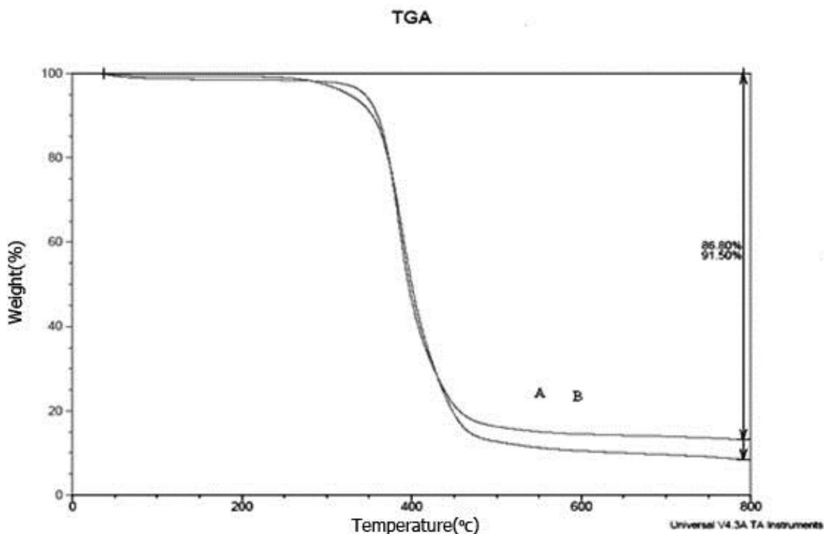
Fig. 11: TGA Curves Epoxy Nanocomposite (Expt.3 and 18).
