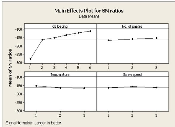
**Fig. 7:** Main Effects Plot for S/N Ratio Values of Surface Conductivity.
