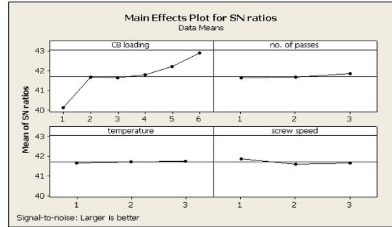
**Fig. 9:** Main Effects Plot for S/N Ratio Values of Glass Transition Temperature.
