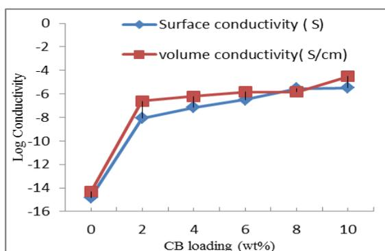
**Fig. 1: Volume and Surface Resistivity for Epoxy/CB Nanocomposites.**
