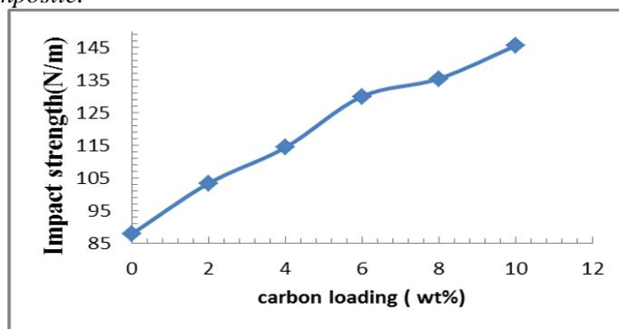
Fig. 5: Impact Strength of Epoxy/CB Nanocomposite.
