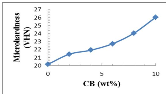
Fig. 3: Microhardness for Epoxy/CB Nanocomposite.
