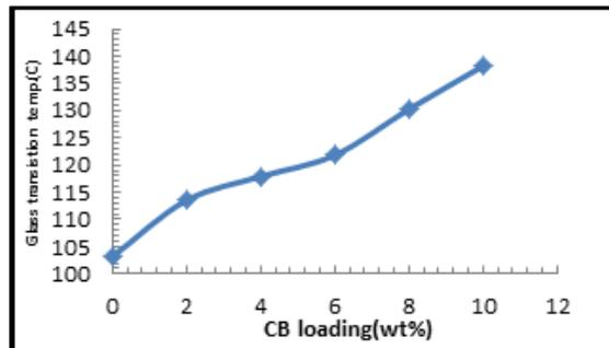
Fig. 4: T<sub>g</sub> for Epoxy/CB Nanocomposite.
