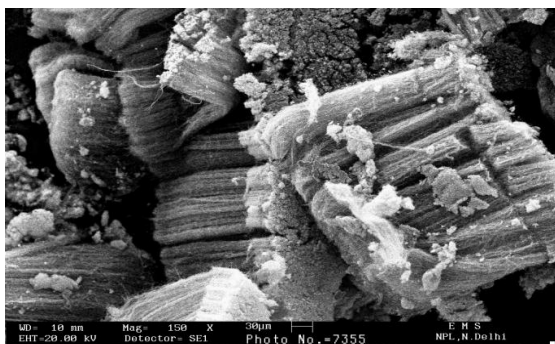
Fig. 1: SEM Image of As-Produced MWCNT Aligned Bundles.
