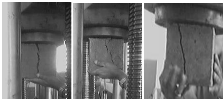
Fig. 5: Cracking pattern of Specimen.
