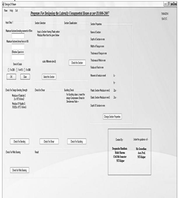
Fig.1: Design of Laterally Unsupported Beam as per IS: 800-2007.
