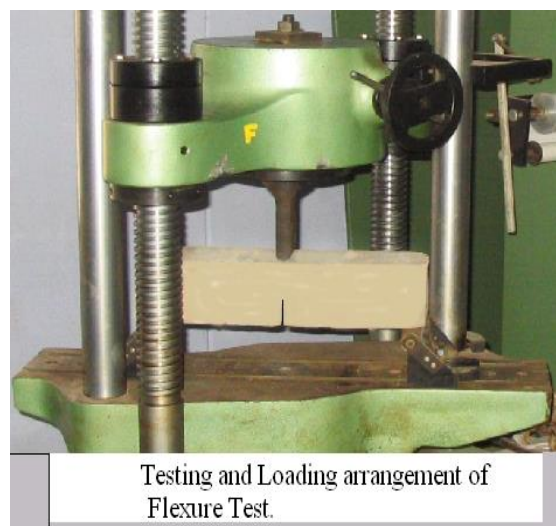
Fig. 5: Testing and Loading Arrangement of Flexure Test.
