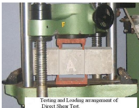
Fig. 3: Testing and Loading Arrangement of Direct Shear Test.
