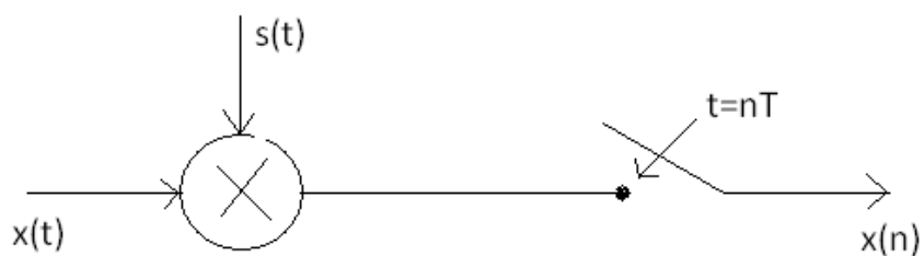
Fig. 1.b: Sampled Sequences x(n) , Sampling of Continuous Time Input Signal x(t) .
