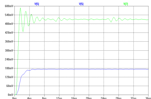
Fig. 12 A Spice Model for Delay Calculation in RLCG Network Using Values R(K\Omega) = 1.2 , L(nH) = 2.7 , C(pF) = 2.4 and G(mS) = 3.0 in a 0.18 \mu m Technology.
