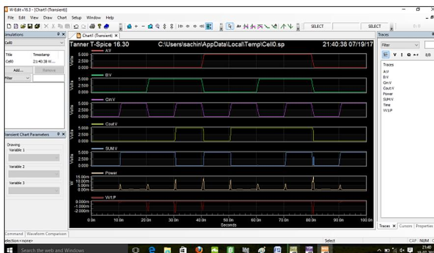
*Fig. 6: Waveform of CMOS Adder Circuit.*
