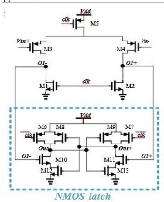
Fig. 1: The Conventional Two-stage Dynamic Comparator [8].
