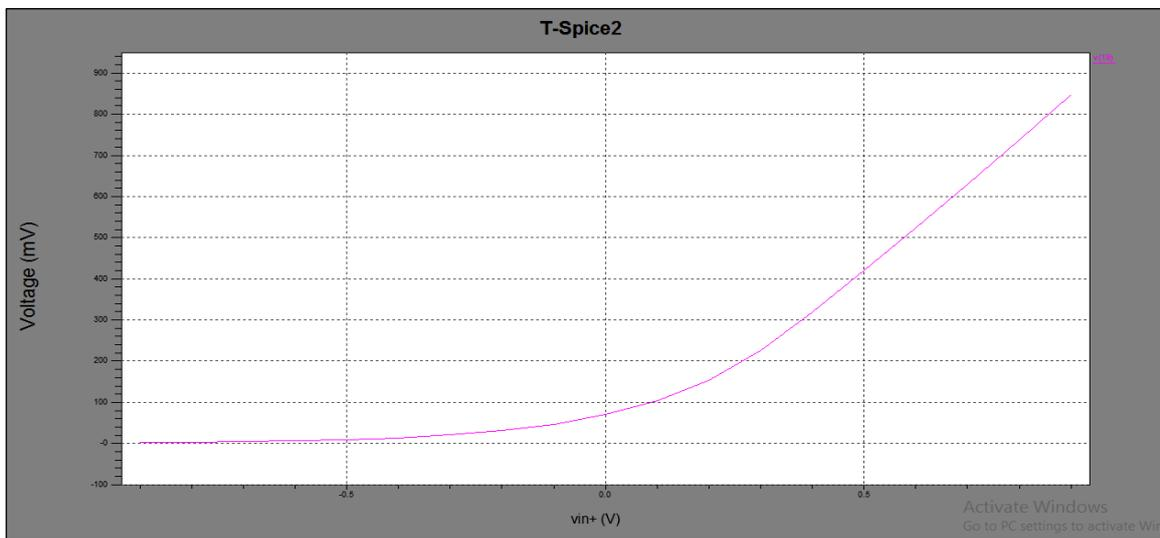
**Fig. 6: ICMR (Input Common Mode Range).**
