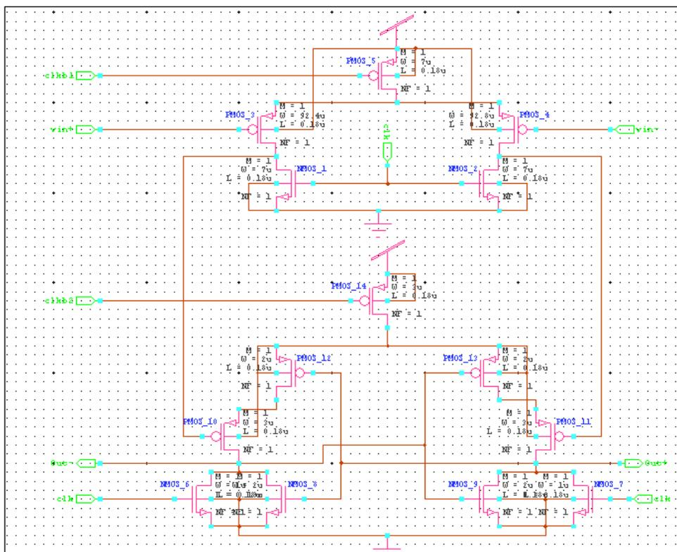
Fig. 2: The Proposed Two-stage Dynamic Comparator.
