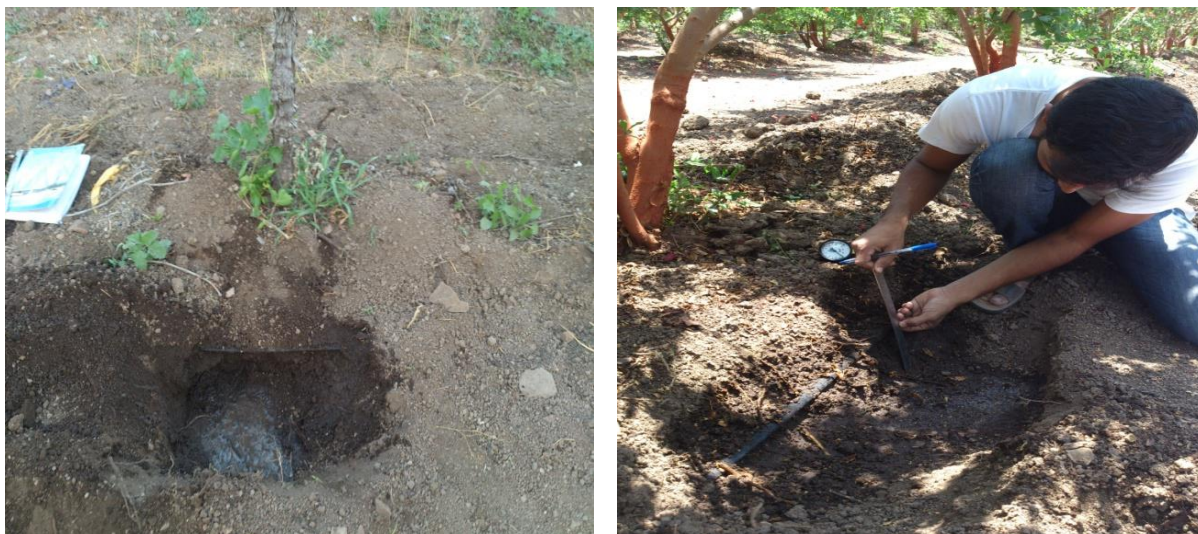
Fig. 3: Wetted Zone below Porous Drip Tube.
