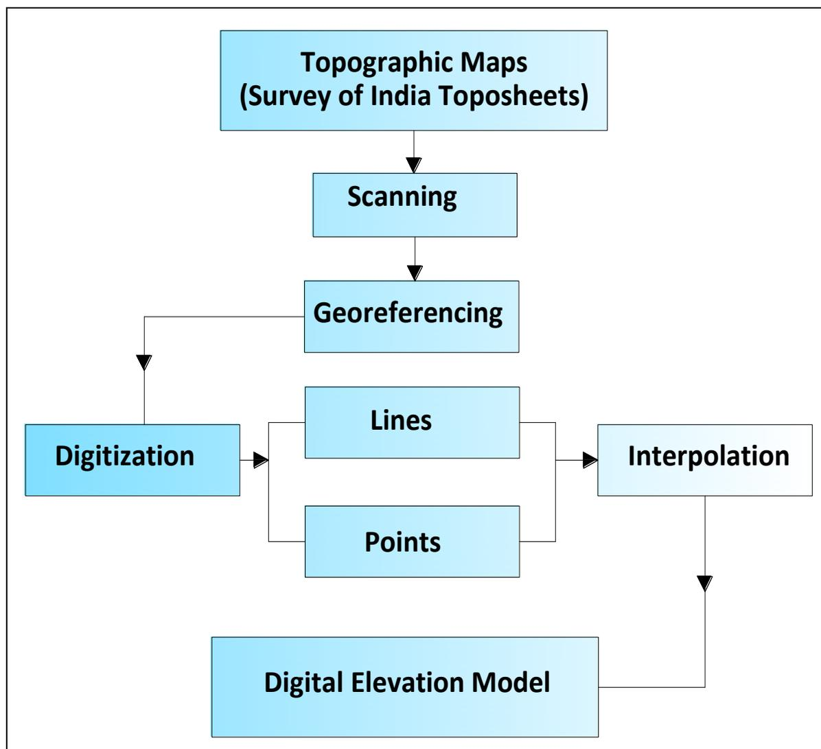
*Fig. 1: Flow Diagram of Creating DEM.*
