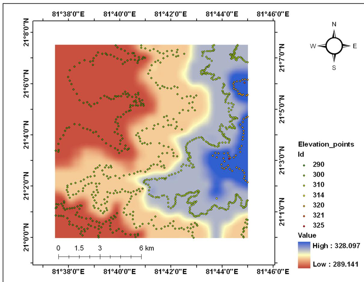
Fig. 6: DEM of Area of Interest using Elevation Points.
