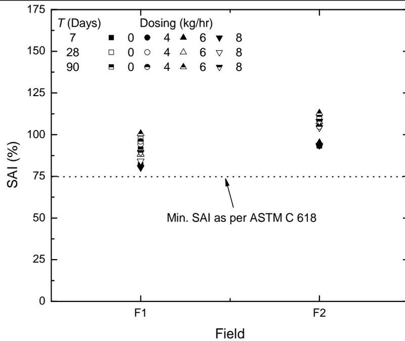
**Fig. 3** Strength Activity Index of Fly Ash Samples
