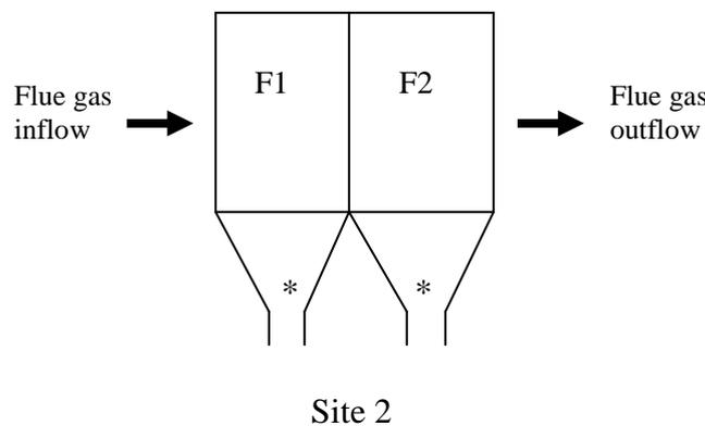
**Fig. 1** Schematic of Sampling Locations in the ESP.
