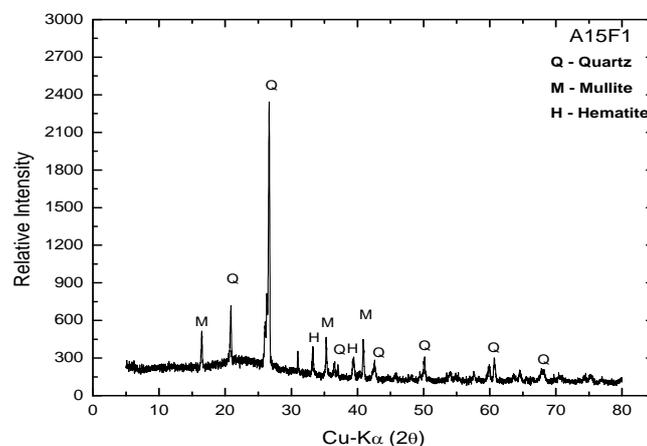
**Fig. 6** A typical X-ray Diffract gram of a Fly Ash Sample
