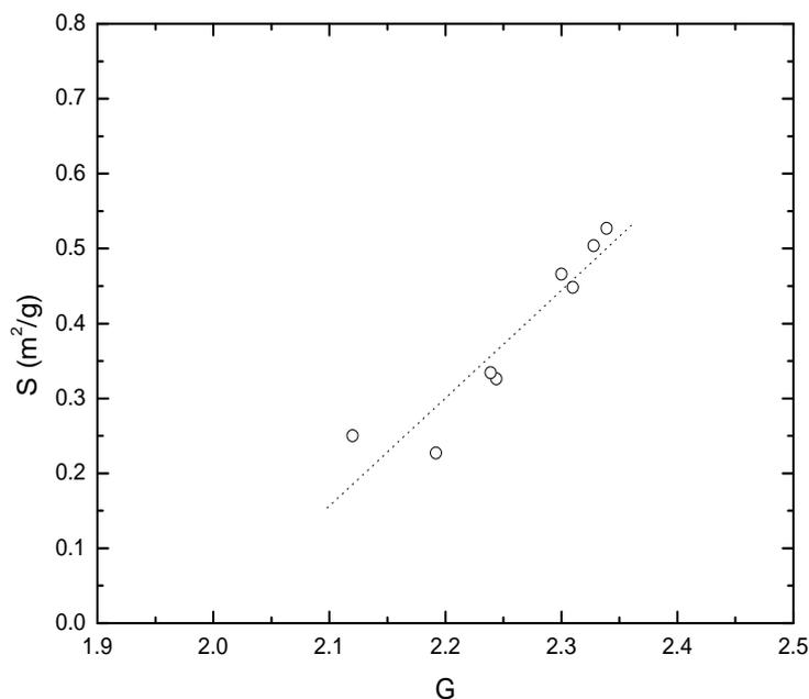
**Fig. 4** The relationship between Specific Gravity and Specific Surface Area of Fly Ashes
