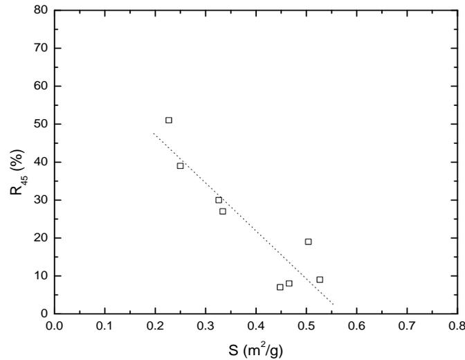
**Fig. 5** The Relationship Between Specific Surface Area and R<sub>45</sub> of Fly Ashes.
