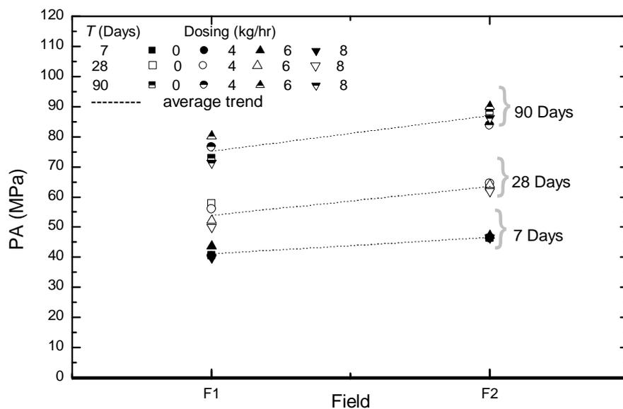
**Fig. 2** Pozzolanic Activity of Fly Ash Samples
