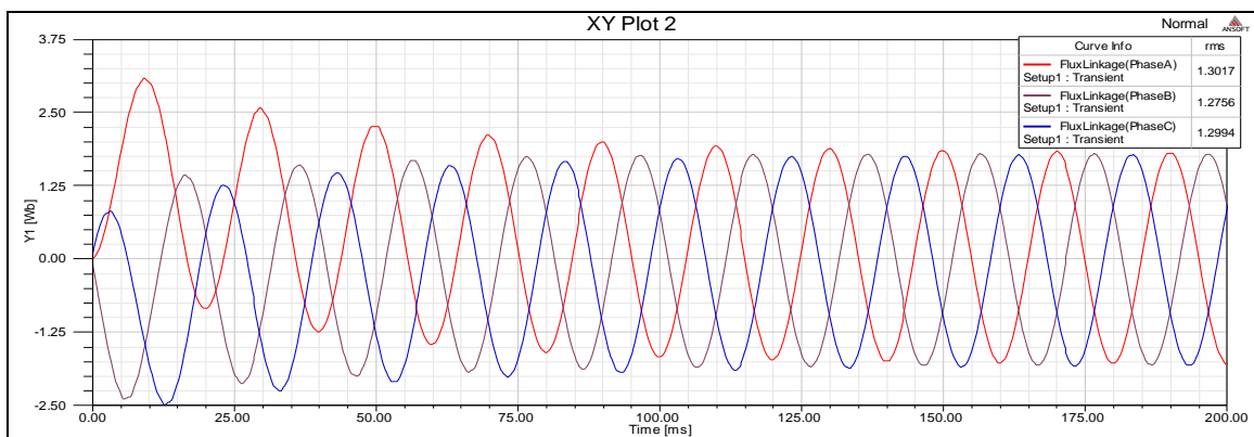
Fig. 6: (e) Flux Linkage Response under Normal Condition.
