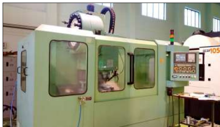
Fig. 3: 3-Axis CNC Machine Used for Machining of the Blade.
