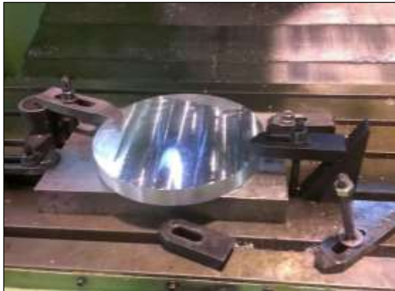
Fig. 10: Raw Material Fixed in CNC Bed.
