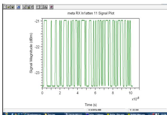
**Fig. 11** Received Optical Waveform at the Distance of 400 m.
