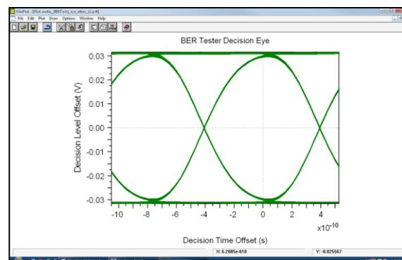
**Fig. 8** Receiver Eye Diagram at the Distance of 50 m.
