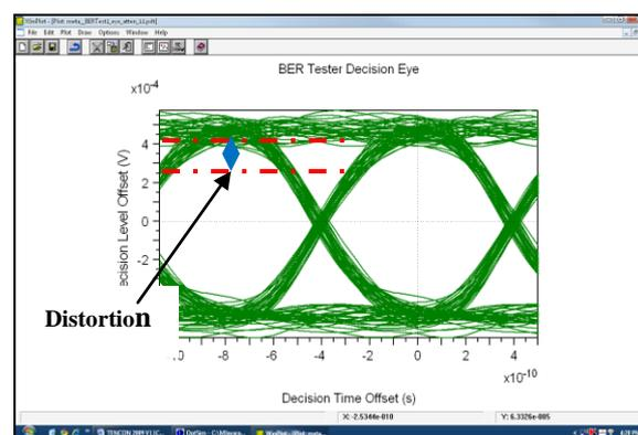
**Fig. 9** Receiver Eye Diagram at the Distance of 400 m.
