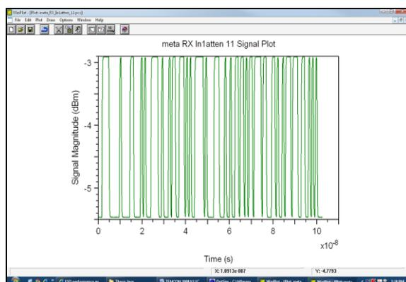
**Fig. 10** Received Optical Waveform at the Distance of 50 m.
