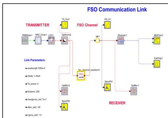
Fig. 3 FSO Block Diagram.
