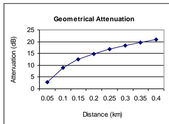
Fig. 5 Geometrical Attenuation for Various Distances.
