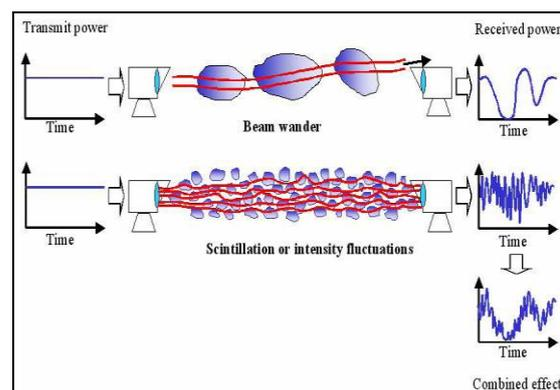
**Fig. 12** Beam Wander and Scintillation Attributed to Atmospheric Turbulence.
