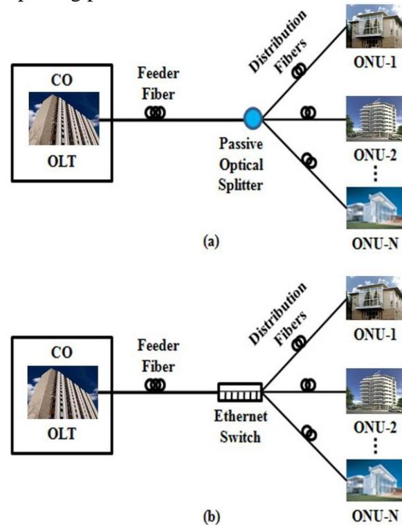
**Fig. 2** Architecture of P2MP Based Optical Networks. (a) Time Division Multiplexed Passive Optical Network (TDM-PON); (b) Active Optical Network (AON).
