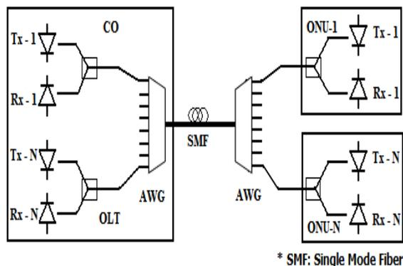
**Fig. 10** Architecture of the Basic WDM-PON.
