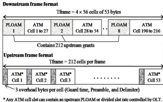
**Fig. 6** Downstream and Upstream Frame Structure of 622/622 Mb/s B-PON [13].
