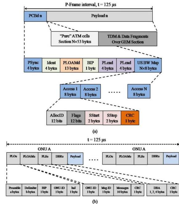
**Fig. 9** Frame structures and overheads of G-PON. (a) Downstream frame structure; (b) Upstream frame structure [14].
