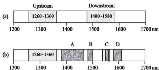
**Fig. 7** Wavelength allocation for A-PON and B-PON. (a) Original spectrum allocation for A-PON; (b) Subsequent allocation for B-PON providing wavelengths for enhancements and other future uses [5].
