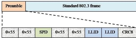
**Fig. 8** Frame Structure of E-PON [14].
